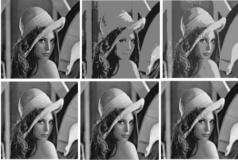
Figure 2: Top left corner: orinal image; left to right: reconstructed Lena image using 2 \times 2 blocks at quality indices 5, 10, 50, 90, 95.
